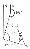
**6.** To find the distance *d* across a pond, a surveyor determined the measurements shown below. How far is it across the pond?
